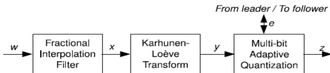
**Fig. 1. Flow chart of high rate uncorrelated bit extraction.**
