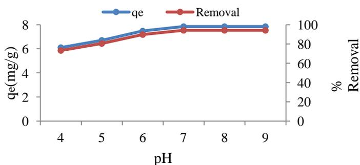
**Fig 1: Effect of pH on Cd(II) adsorption. (C 0 = 25 mg/L, time = 90 min, temp= 25 ± 2° C and dose=3 g/L).**
