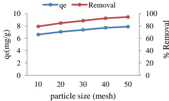
**Fig 2: Effect of particle size on Cd(II) adsorption. (C<sub>0</sub> = 25 mg/L, time = 90 min, temp= 25 ± 2° C and pH=7).**
