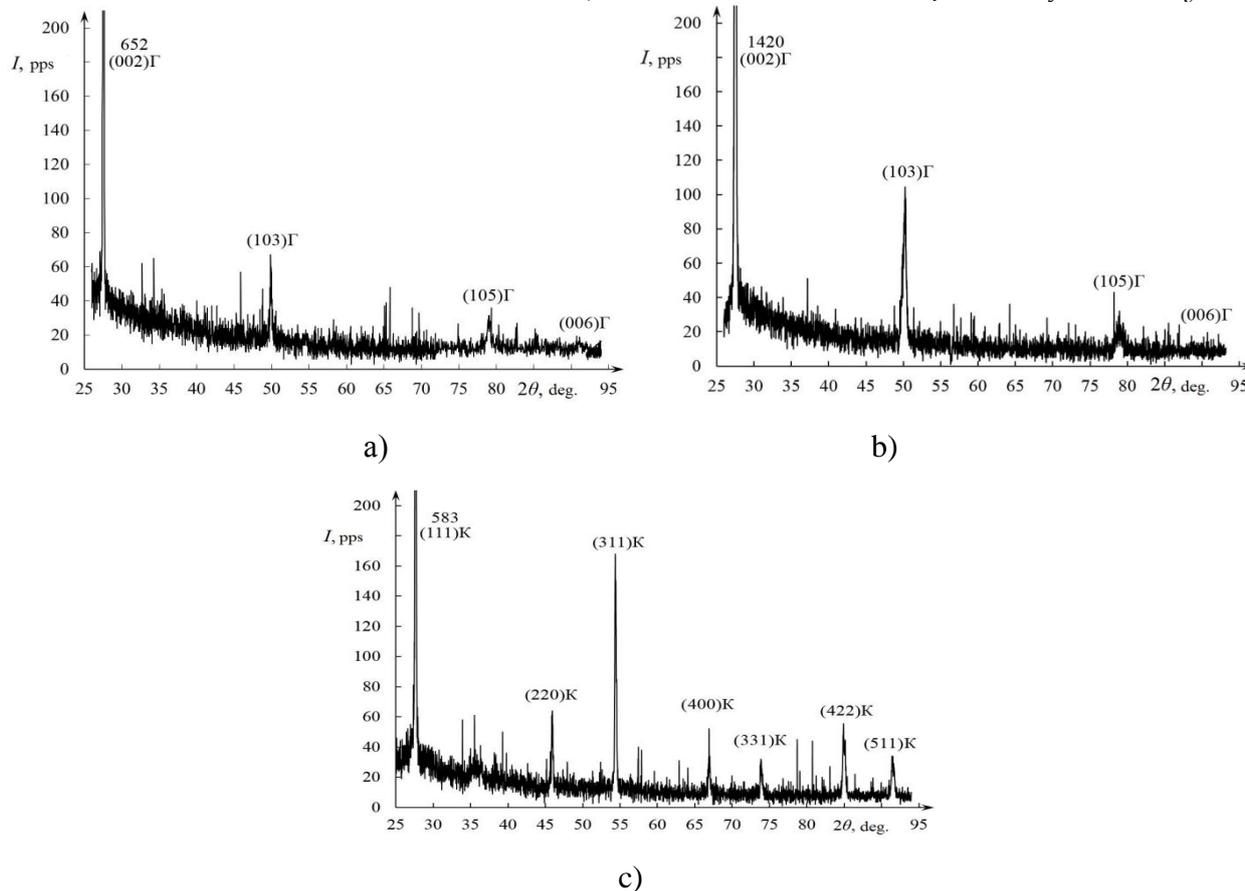
**Figure 2 - X-ray diffractograms of CdTe films:**
