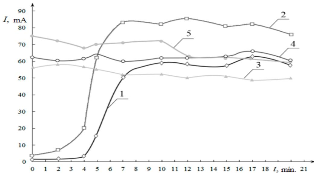
Figure 1 - The discharge current dependence on the sputtering time for various processes.
