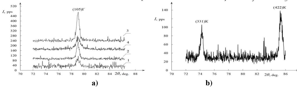
**Fig. 3- X-ray patterns for basic CdTe layers during the "oblique" shooting:**
