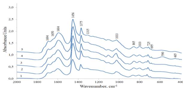
Figure – IR spectrums of initial bitumoid (1) and test products: 2 - product of non-catalytic aquathermolysis (150 °C); 3 - product of non-catalytic aquathermolysis (200 °C); 4 - product of catalytic aquathermolysis (150 °C); 5 – product of catalytic aquathermolysis (200 °C).
