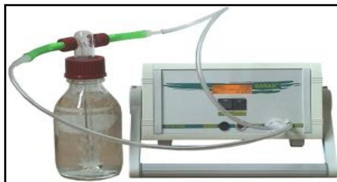
**Figure-2: The measurement concentration of radon 222 by radon meter device model RTM1688-2.**
