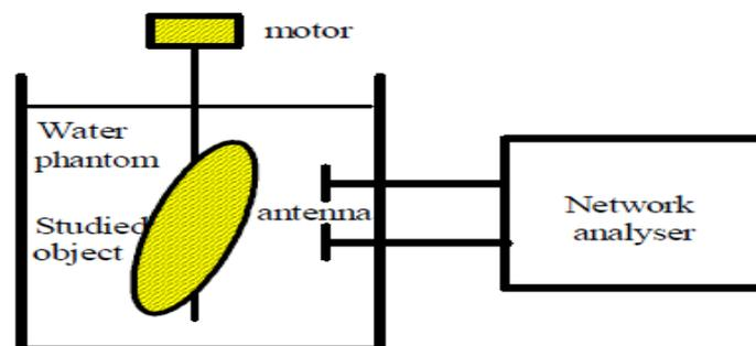
**Fig. 3. Schematics of experimental setup of microwave tomograph for biomedical imaging**
