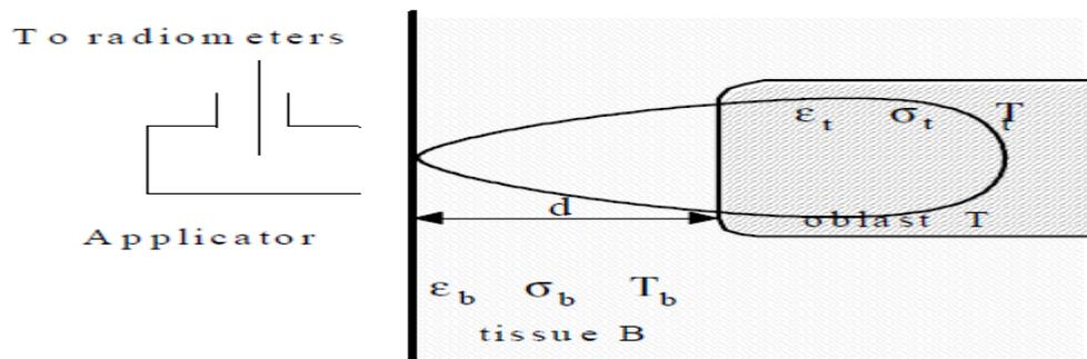
**Fig.4: Principals of imaging by a microwave radiometer.**
