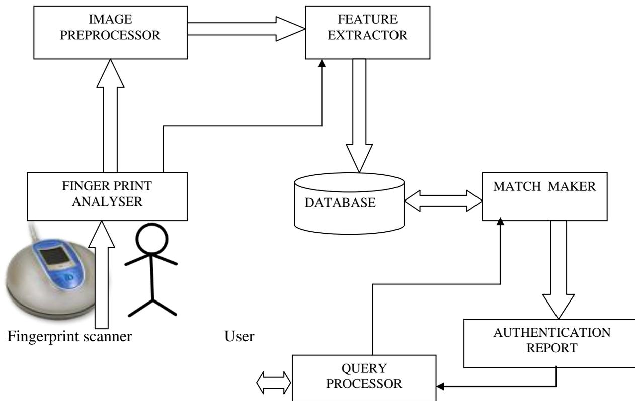
**Figure 1: Architecture a general-purpose fingerprint matching system.**
