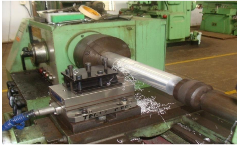
Figure-2: Double Point Cutting Tool does Turning on Aluminum bar.
