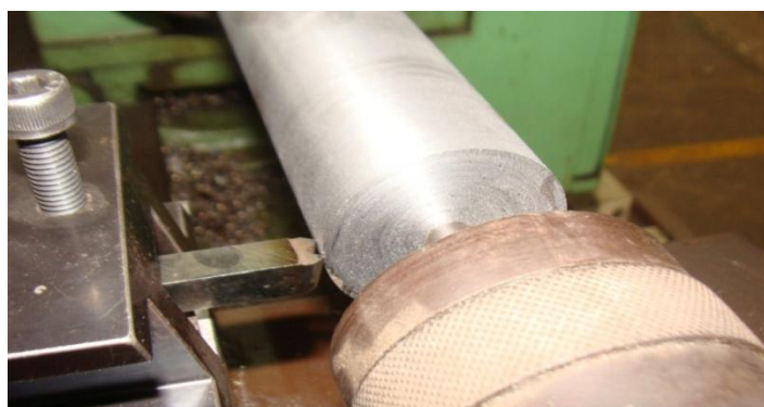
Figure-1: HSS Double Point Cutting Tool has been fixed in the tool post for turning on Aluminum Bar.
