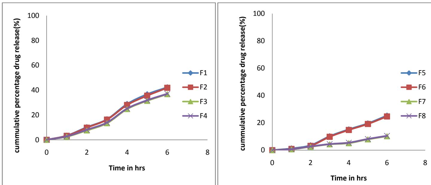
Figure: 4 In-vitro dissolution profile of Olsalazine sodium optimized formulation F6 after enteric coating with Eudragit –S 100.
