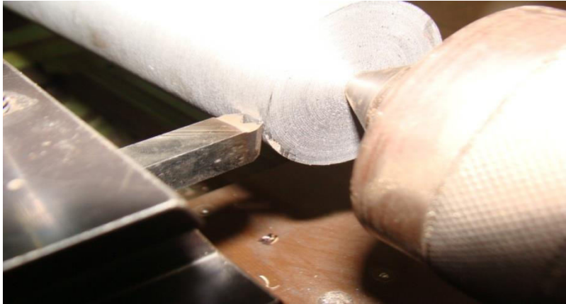
Figure -1: HSS Double Point Cutting Tool for turning on Aluminum Bar.
