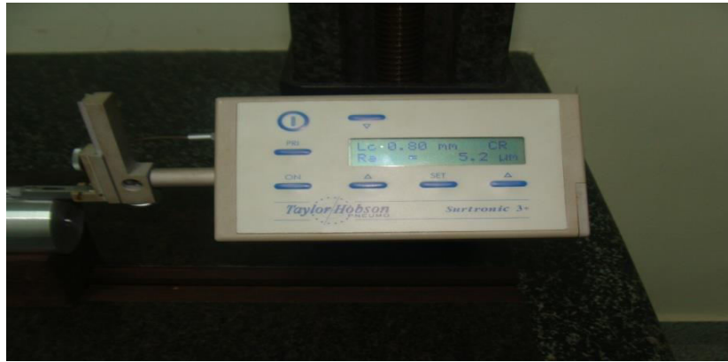
Figure-3: Taylor-Hobson Surtronic 3+ Surface Roughness Measuring Instrument.
