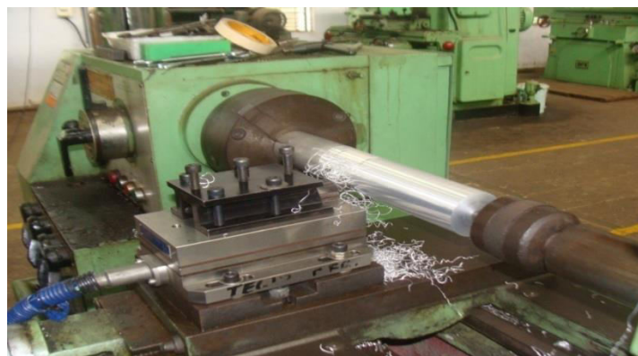
Figure-2: HSS Double Point Cutting Tool does turning on Aluminum Bar.
