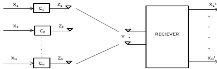
**Fig. 2 Block diagram of Orthogonal CDMA access scheme over Block fading MIMO MAC**
