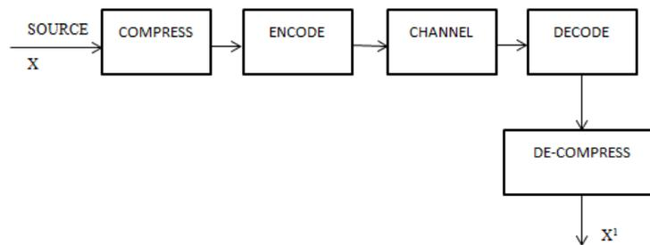
**Fig. 1. Block diagram for Joint Source Channel Coding**
