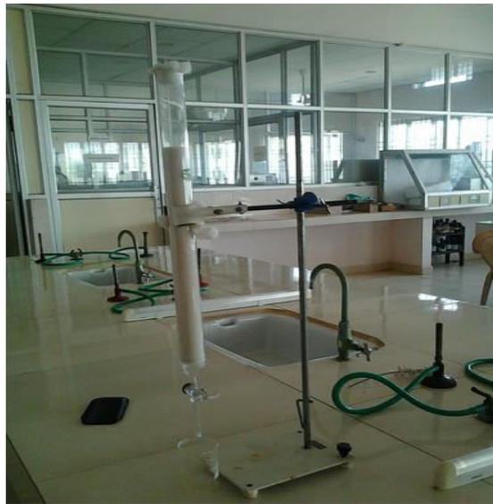
**Figure 7: Preparation of column.**
