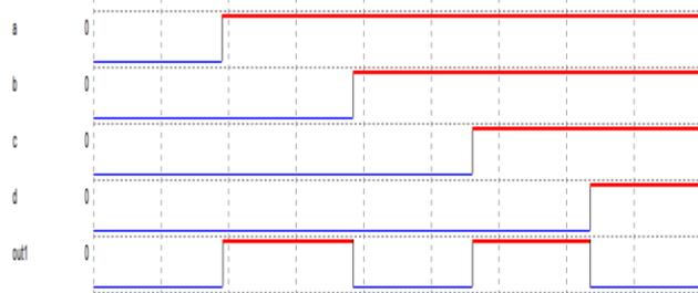
**Fig. 14. Verification of the parity checker using timing diagram.**
