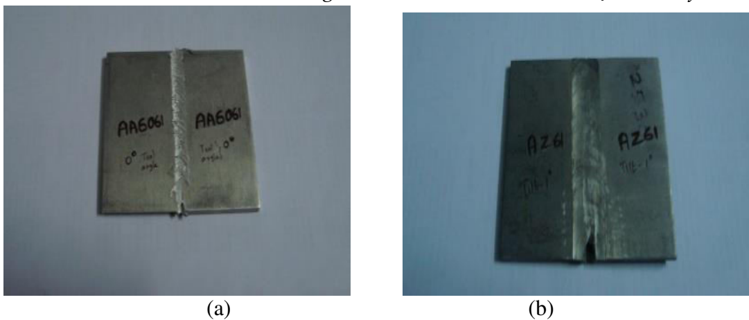
Fig.1 Friction Stir Welding of Similar alloys: (a) AA6061-AA6061 (b) AZ61-AZ61.
