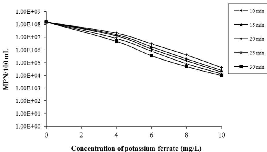
Figure.6. MPN /100 ml at the various dosage and contact time in pH of 8.
