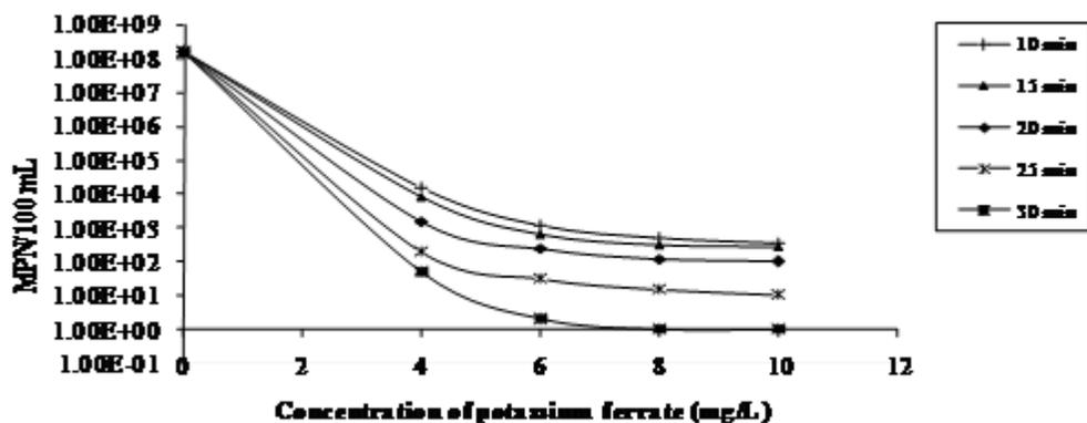
Figure.4. MPN /100 ml at the various dosage and contact time in pH of 6.
