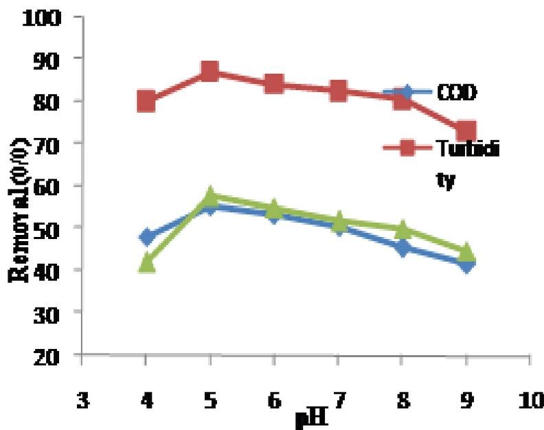
Figure.1. Determination of optimum pH for potassium ferrate in COD, turbidity and phosphorus removal.
