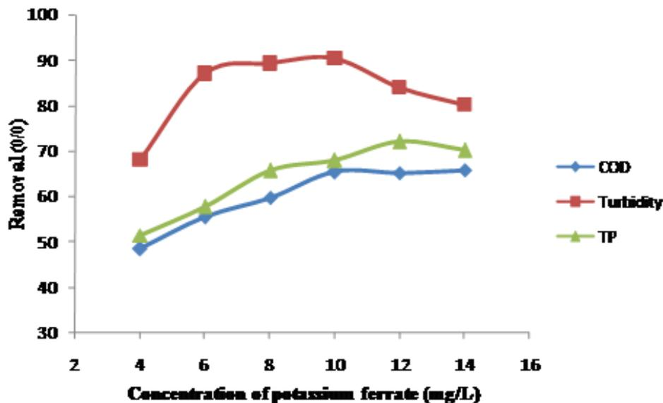
Figure.2. Determination optimum potassium ferrate dosage for COD, turbidity and phosphorus removal.
