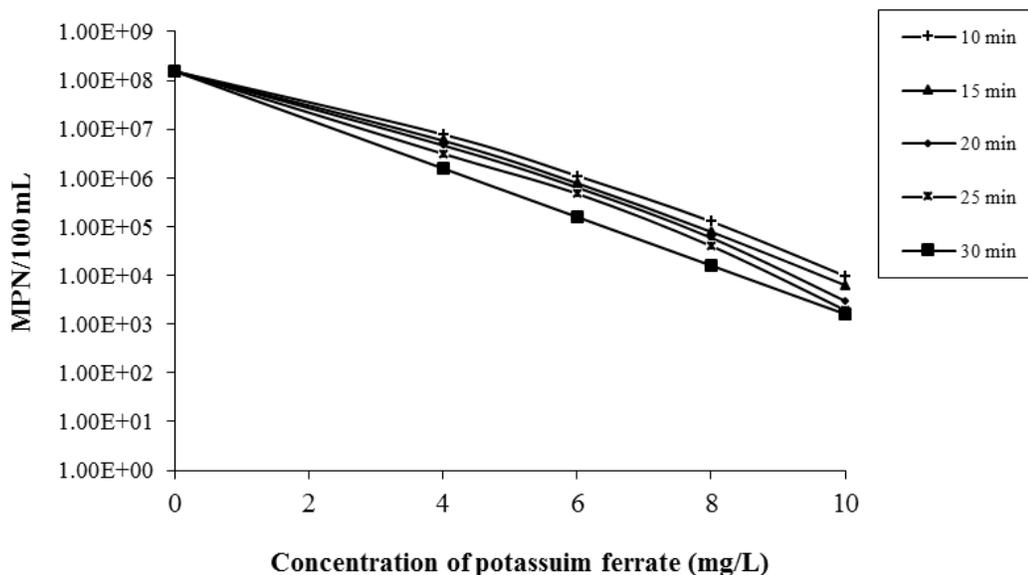
Figure.5. MPN /100 ml at the various dosage and contact time in pH of 7.
