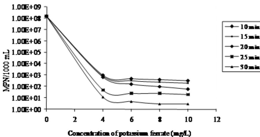
Figure.3. MPN /100 ml at the various dosage and contact time in pH of 5.
