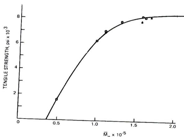
**Fig.1 Molecular wt. versus Tensile strength**
