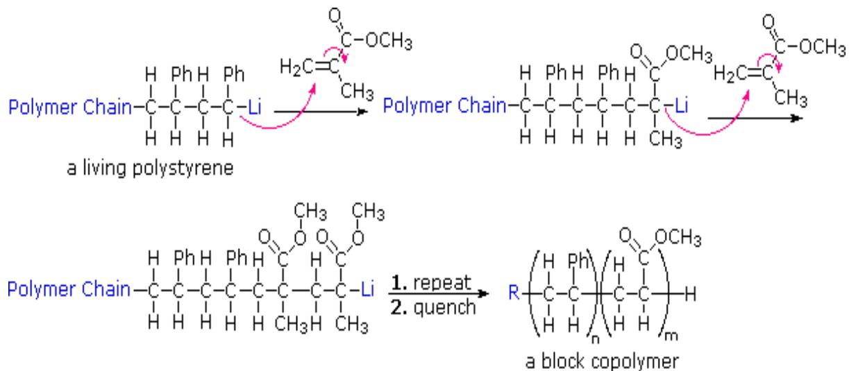
**Fig.9: Block Copolymerization.****Step Growth Polymerization**
