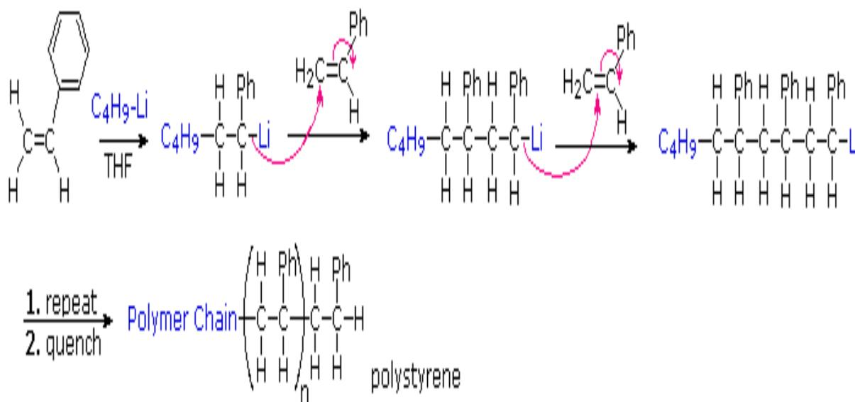
Fig.7: Anionic Chain-Growth Polymerization
