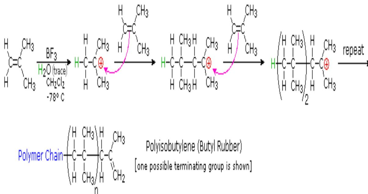
**Fig.6: Cationic Chain-Growth Polymerization:**
