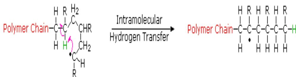
**Fig.5: Chain transfer reaction.**
