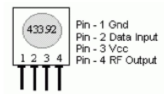
These RF Products are ideal for short-range remote control applications where cost is a primary concern. These modules require no external RF components except for the antenna. They generate virtually no emissions, making FCC and ETSI approvals easy.
