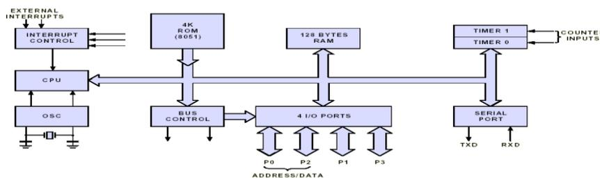
**Block Diagram of the 8051 Core**
