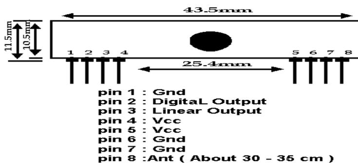
The receiver also operates at 433.92MHz, and has a sensitivity of 3uV. The WS-434 receiver operates from 4.5 to 5.5 volts-DC, and has both linear and digital outputs. A 0 volt to Vcc data output is available on pins. This output is normally used to drive a digital decoder IC or a microprocessor which is performing the data decoding. The receiver's output will only transition when valid data is present. In instances when no carrier is present the output will remain low.
