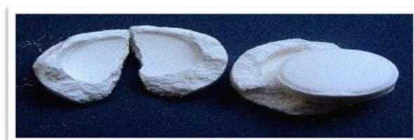
Fig 1.2: Equatorial fracture showing the surfaces of the compressed ethyl cellulose core tablet system.
