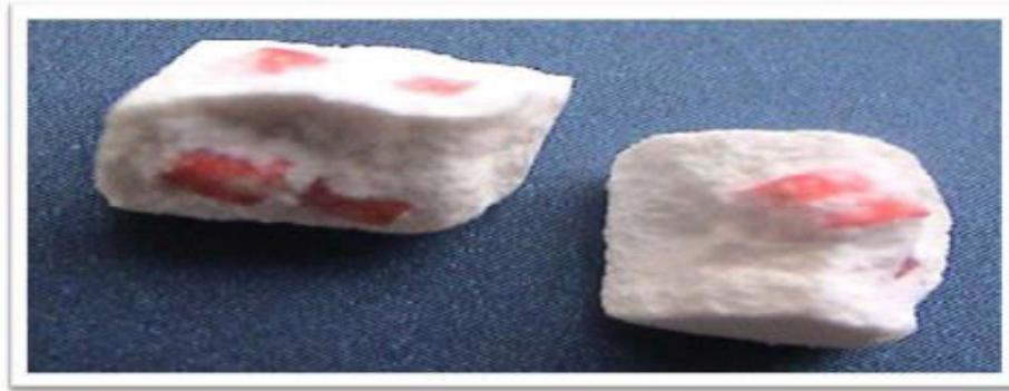
Fig 1.4: Fracture equatorial showing surfaces of the compressed mini-tablets system
