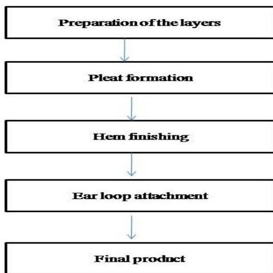
Figure 1: Development of dual Ply mask.
