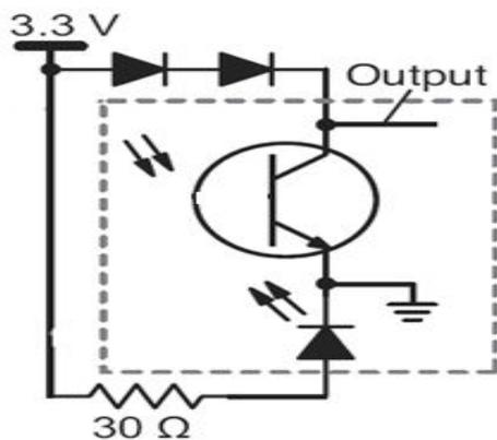
Fig-1: Sensor circuit- Schematic diagram of reflective photosensor.
