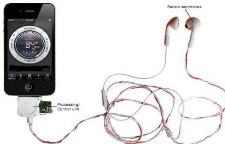
**Fig-3: Prototype of earphone system with reflective photosensor.**
