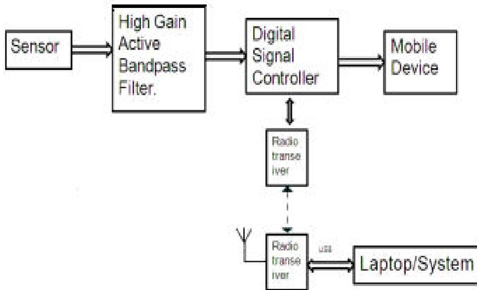
**Fig-2: Overview of the system architecture.**
