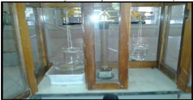
Fig-1: Modified physical double beam balance for Invitro Bioadhesive strength.
