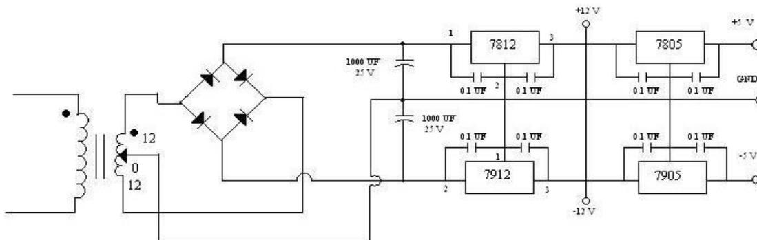
**Fig 2: Power supply block.**
