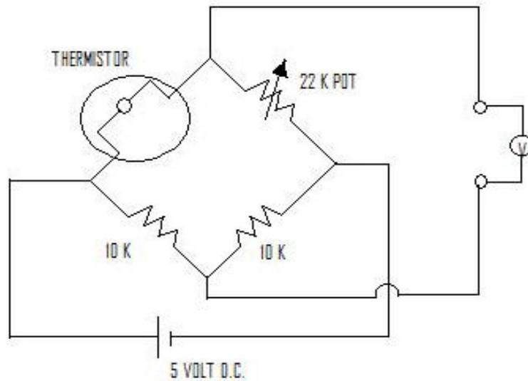
**Fig 3: Temperature Sensing Circuit (Blood bag).**
