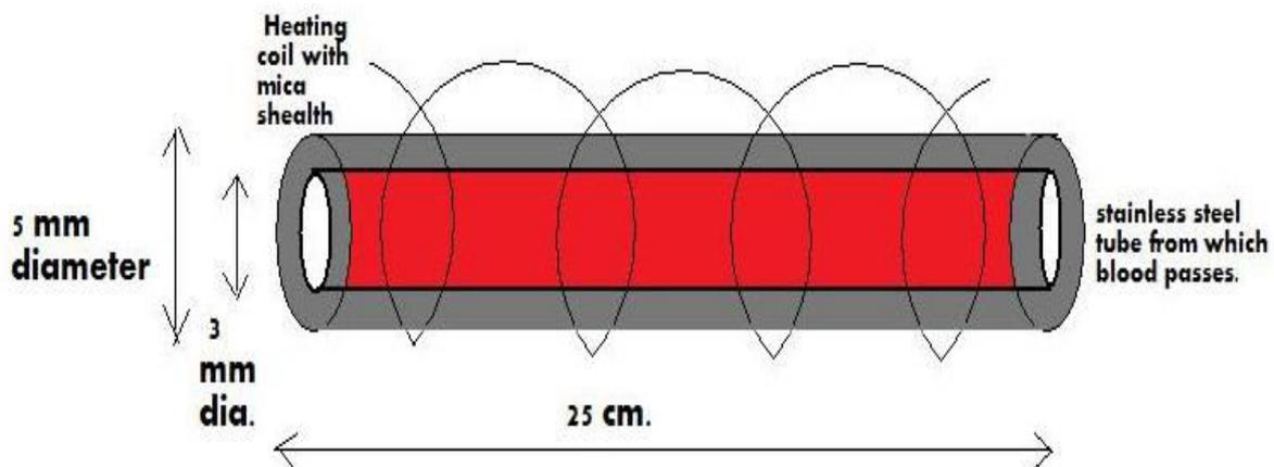
**Fig 9: Heating Element.**
