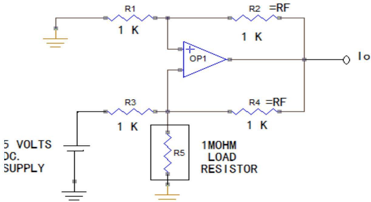
Fig 8: Voltage to Current Converter Circuit.
