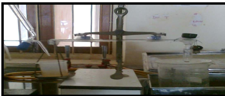
Figure-1: Schematic representation of modified physical balance for bioadhesion strength measurement
