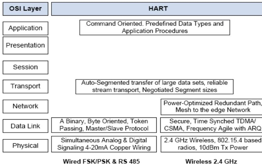
Fig. 2 Architecture of HART Communication Protocol [13]
