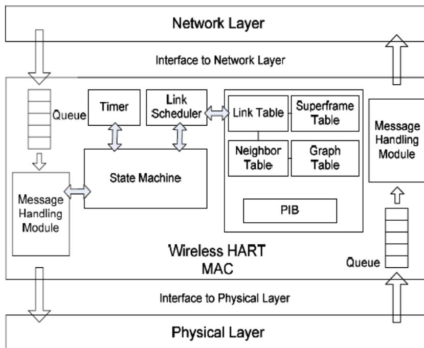
Fig. 3 Wireless HART Data Link Layer Architecture [13]
