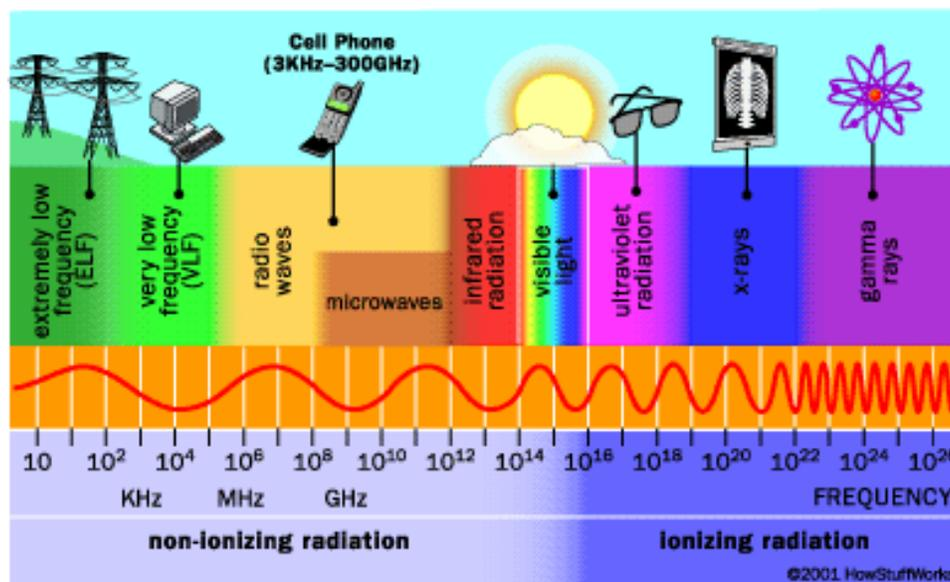
**Fig. 1 Typical radio frequencies (RF) for various applications.**
