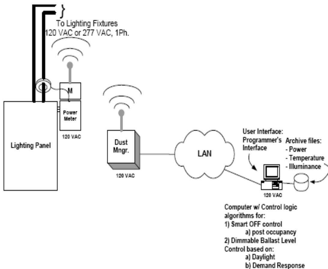
Fig. 4 Schematic illustration of wireless lighting control system.
