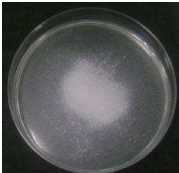
Fig 06 Complete dispersion of tablet at 16 secs
