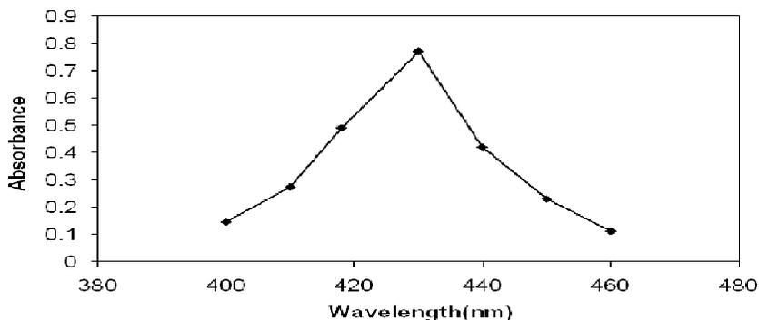
**Absorption spectrum of LST with SBT/ $CHCl_3$  system**
