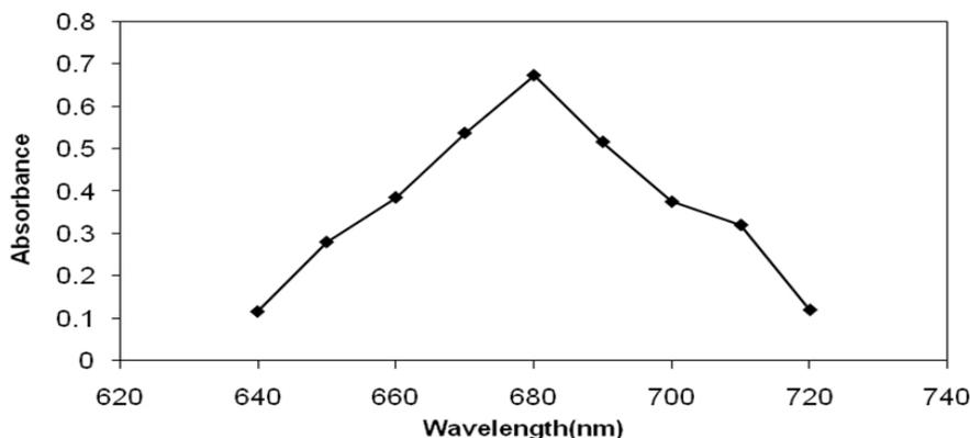
**Absorption spectrum of LST with  $K_3Fe(CN)_6/FeCl_3$  system**
