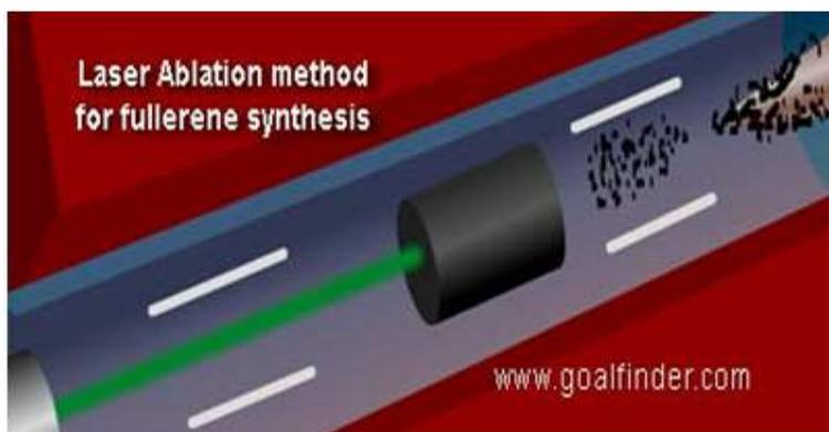
**Fig.7. Diagrammatical representation of laser ablation setup for synthesis and growth of nanotube.**
