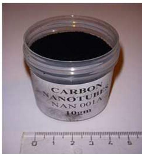
**Fig.3. Powder of carbon nanotube.**
