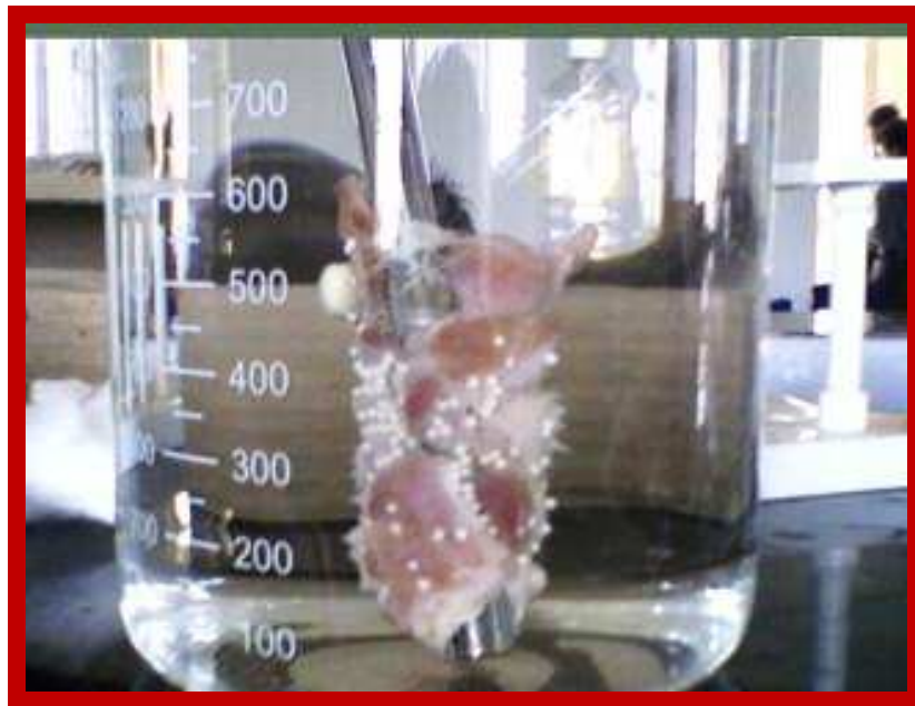
Figure - 02: In vitro wash-off test of microcapsules.
