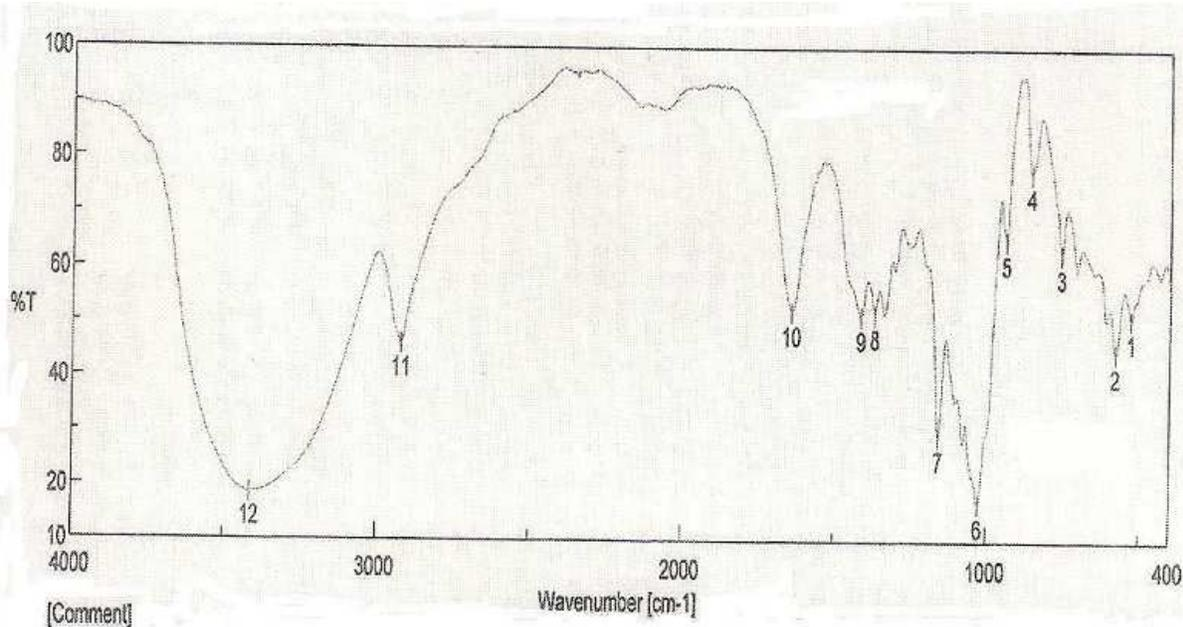
**Fig. 3. FTIR spectra of  $\beta$ -cyclodextrin.**
