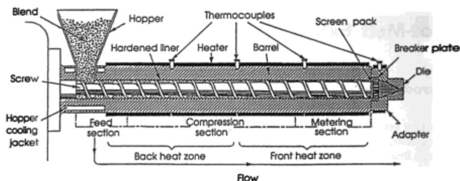
**FIG. 1.** Schematic diagram of a single screw extruder
