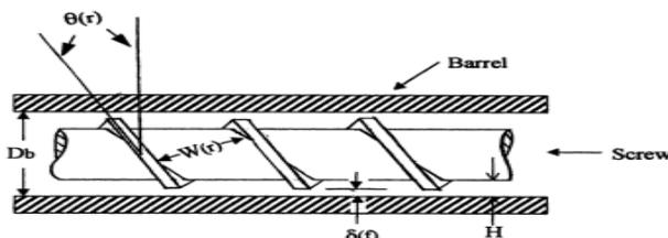
**FIG. 2.** Geometrical diagram of an extruder screw. Diameter of the barrel ( $Db$ ) = inside diameter of the barrel; channel depth ( $H$ ) = distance from screw roots to barrel inner surface; flight clearance ( $\delta(r)$ ) = the distance in between the flight and the barrel inner surface; channel width ( $W(r)$ ) = distance in between two neighboring flights; helix angle ( $\theta(r)$ ) = angle formed in between the flight and the direction perpendicular to the screw axis.
