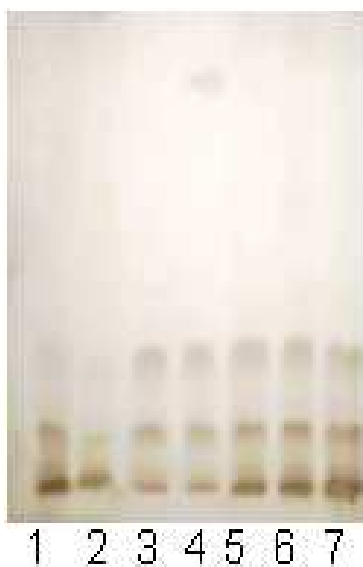
Fig. 3: HPTLC Plate image at visible light developed with Vanillin-Sulphuric acid Reagent. 1&2: Arogyawardhini Bati methanolic extract (50 \mu l), 3 & 4- methanolic extract of P.kurroa (20 \mu l), 5-7: methanolic extract of Arogyawardhini Bati and Picrorhiza kurroa (50 + 20 \mu l).
