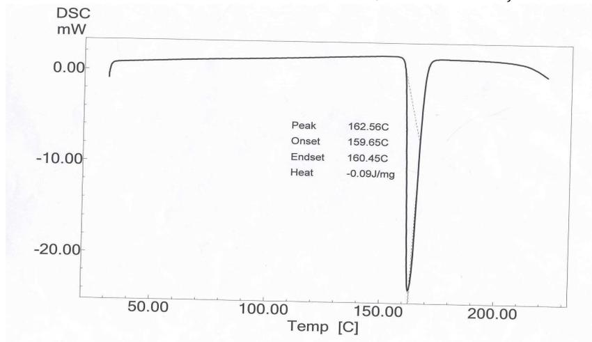
**Fig. 1. DSC Thermogram of pure Metronidazole.**
