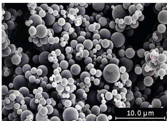
**Figure 1: SEM photomicrograph of uncoated microspheres.**
