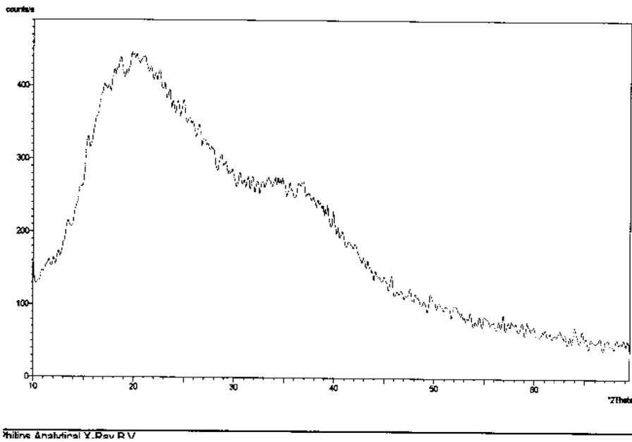
Figure 10: XRD Patterns of Carbopol934.
