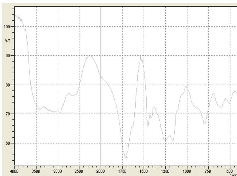
**Figure 4: FTIR peaks of Carbopol934**
