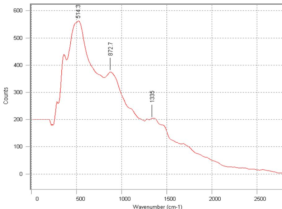
Figure 7: Raman Shifts of Carbopol934.
