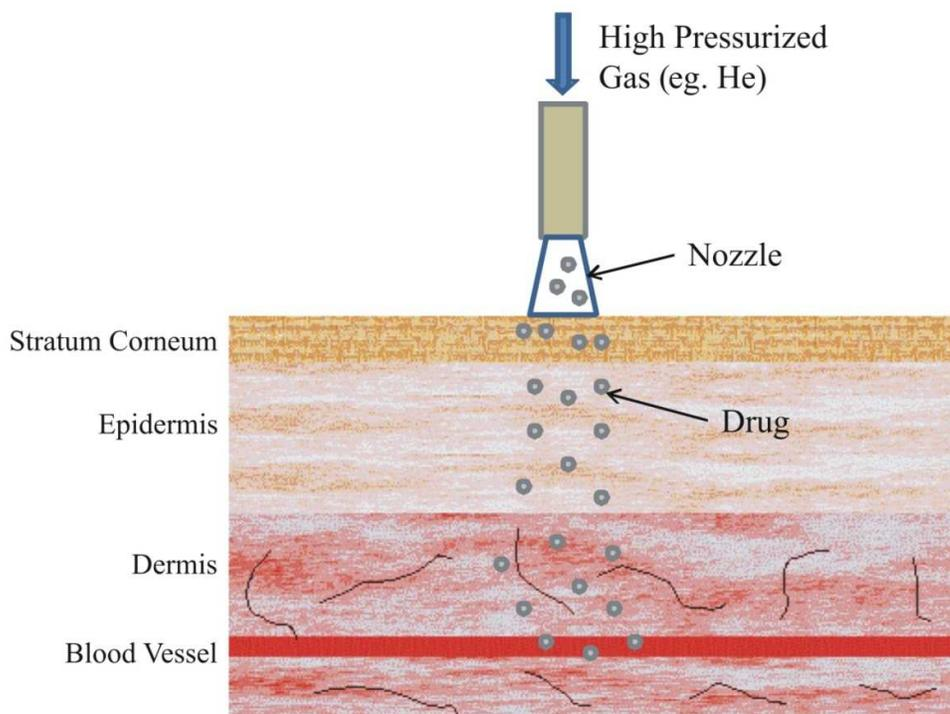
**Fig-2: Jet Injector**
