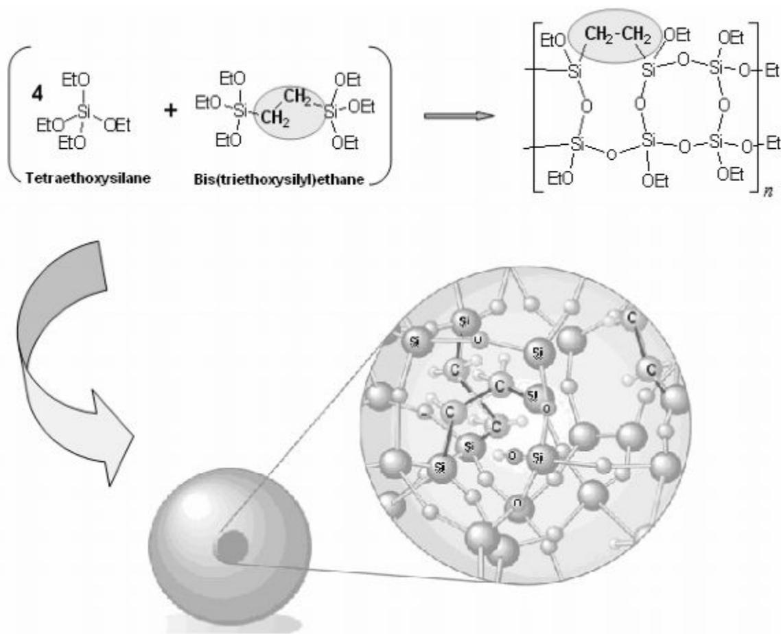
**Figure5: Structure of second generation X-Terra particles.**
