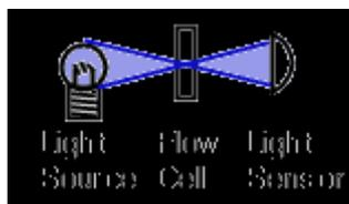
**Fig 4: Variable Wave length detector**
