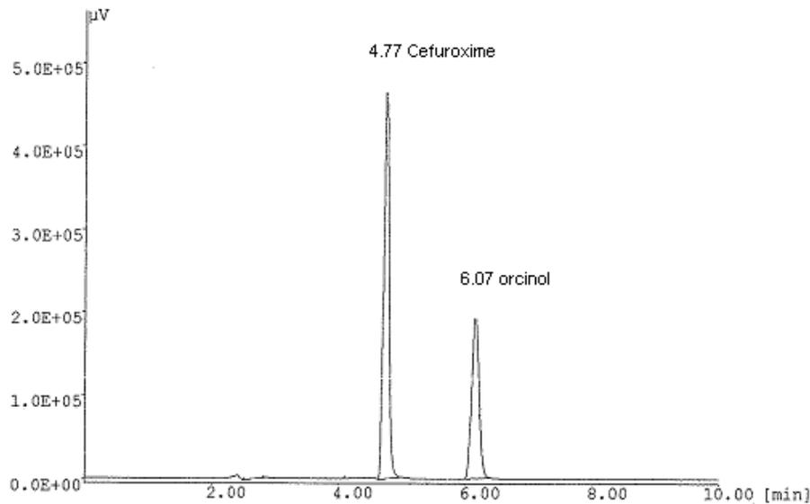
**Figure-4: A typical HPLC chromatogram of the injection containing cefuroxime sodium and orcinol as an internal standard.**
