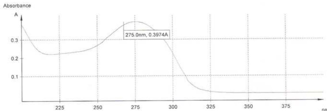
**Figure-2: UV Spectrum of cefuroxime sodium ( $\lambda_{\max}$  determination).**
