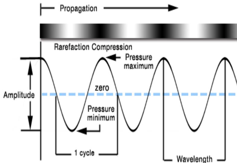
Fig.1: shows a schematic representation of wave propagation<sup>21</sup>
