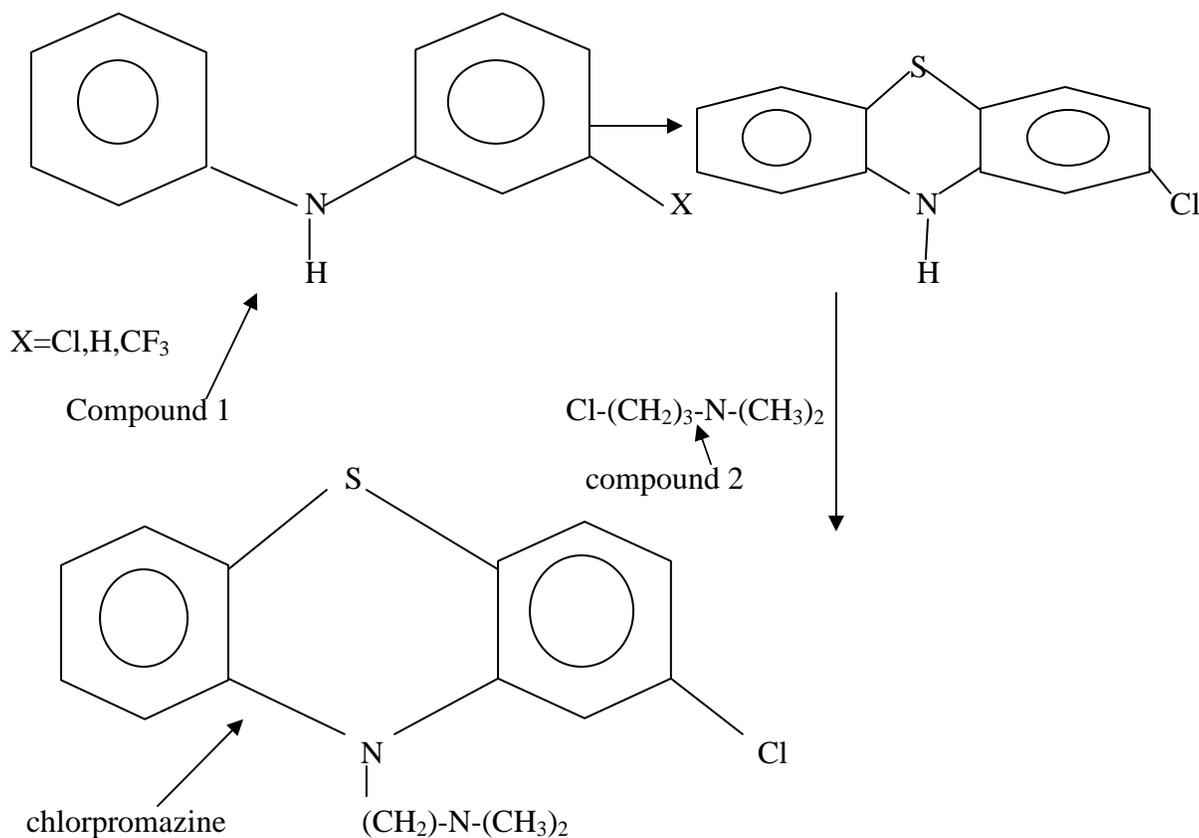
Figure 19: Synthesis of chlorpromazine
