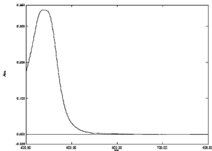
**Figure 2. Visible Absorption Spectrum of Rifaximin (20 µg/ml) in water ( $\lambda_{\max}$  437nm) [Method A]**
