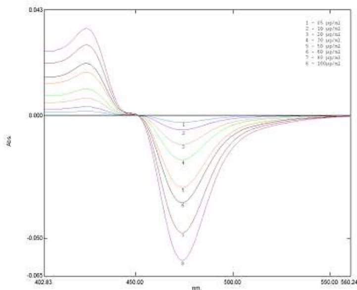
**Figure 3. First Derivative overlain spectra of Rifaximin in Methanol (Minima at 474nm) [Method B]**
