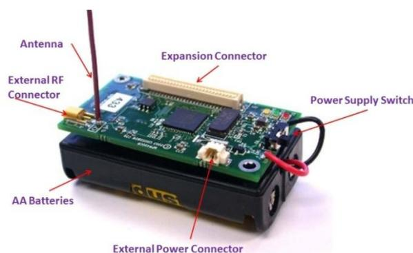
**Figure 3: A simple Sensor node Hardware elements.**
