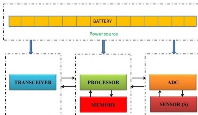
**Figure 2: Single node Architecture.**
