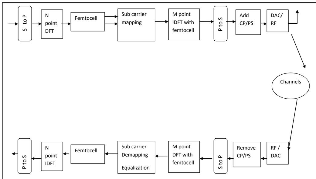
**Fig 1. Transmitter and Receiver Structure of LP-OFDMA/SC-FDMA.**
