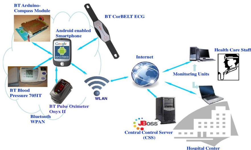
**Figure 2: Wireless Body Area Sensor Network.**
