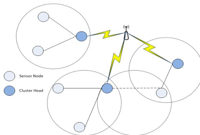
**Figure 3: Cluster Head Selection for Relaying**
