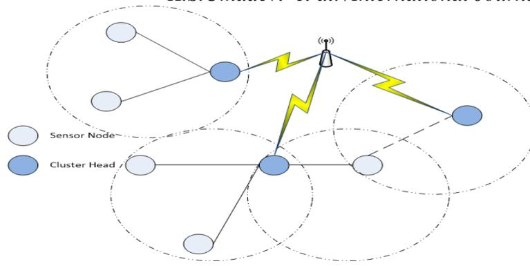
**Figure 4: Change in Cluster Head Selection for Relaying.**
