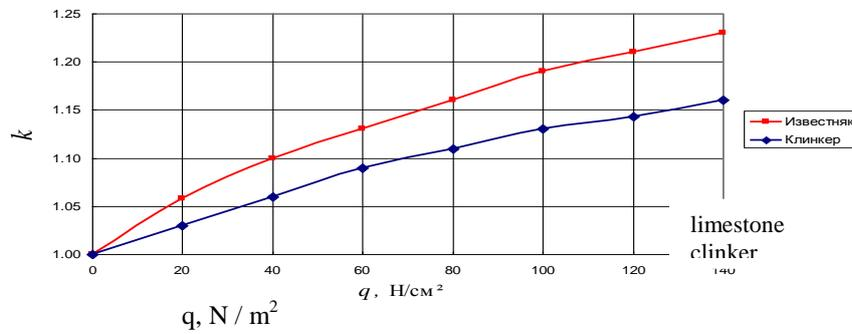
**Figure 5: Dependence of the seals  $k$  on the specific load  $q$**
