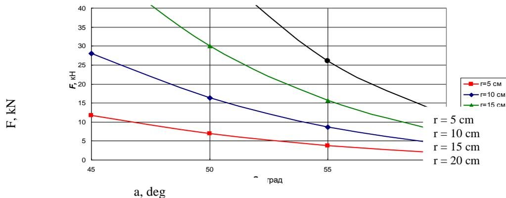
**Figure 7: Dependence of force  $F$  on angle  $\alpha$  for various values of  $r$**
