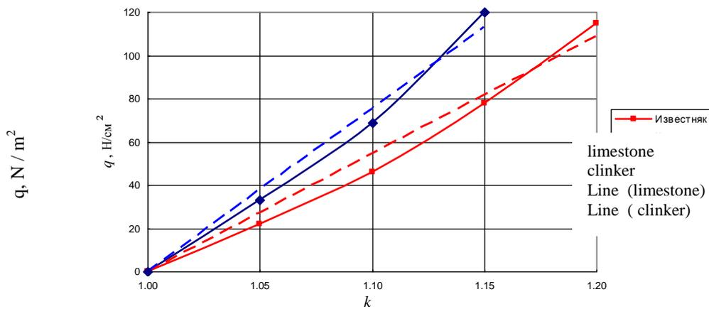
**Figure 6: Dependence of the specific load  $q$  of compaction factor  $k$**
