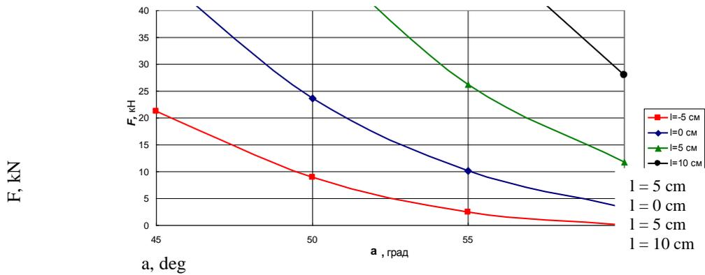
**Figure 8: Dependence of force  $F$  on angle  $\alpha$  for various values of  $l$**
