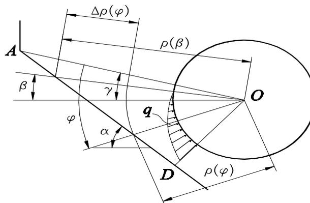
**Figure 4: To the calculation of the intensity of a distributed load  $q$**
