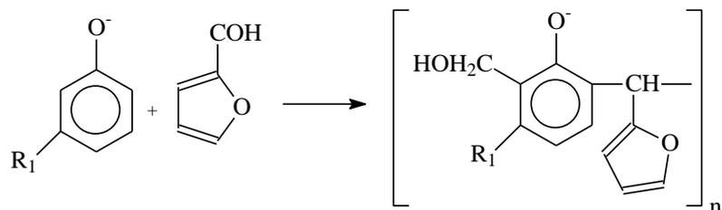
Instead, of СБ-4 superplasticizer scheme obtaining we will present only the empirical formula, because synthesis is possible without condensation stage.
