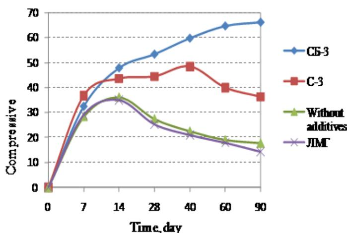
**Fig. 2. Cement specimen durability change in time with various additives (samples were contaminated with mold spores).**
