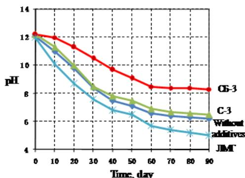
**Fig. 3. Aqueous concrete extract pH change dependence over time.**
