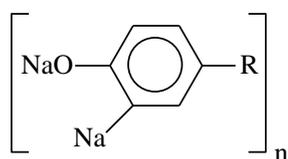
All obtained oxyphenolic supplements are the plasticizing ones in accordance with the GOST 24211-2008. СБ-2A and СБ-4 are related to plasticizers, and СБ-3 СБ-5 are related to superplasticizers [2,3]. They are not inferior to well-known domestic and foreign counterparts according to plasticizing activity.
