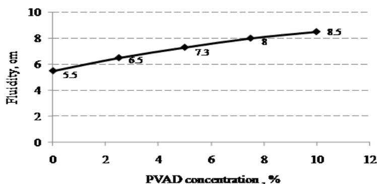
**Fig. 1. The mobility of polymer-cement mixture depending on PVAD concentration.**
