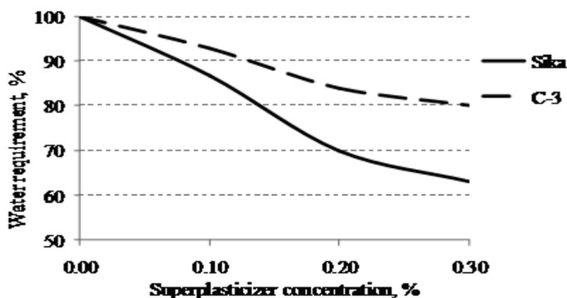
**Fig. 2. The effect of superplasticizers on the water demand of the polymer compound**
