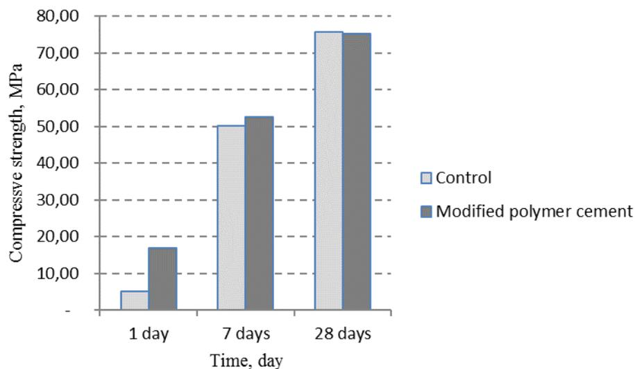
**Fig. 3. Strength indicators of nanomodified polymer cement and cement stone.**
