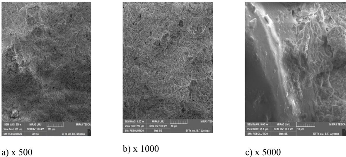
**Figure 2 – micro-structure of powdered concrete on basis of fine-grounded quartzite-sandstone.**
