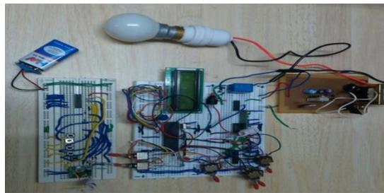
**Figure 8.** Appliances controller setup.
