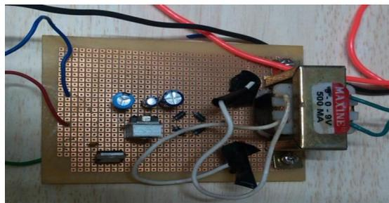
Figure 4. Regulated power supply
