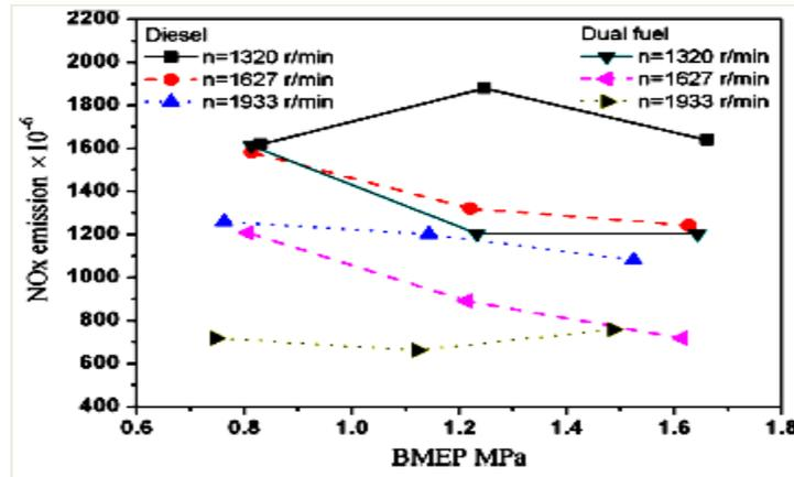
**Fig. 2.NO<sub>x</sub> emission characteristics.**
