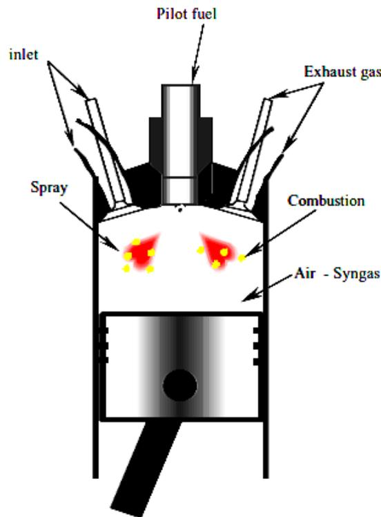
**Fig.3. Concept of dual fuel engine.**
