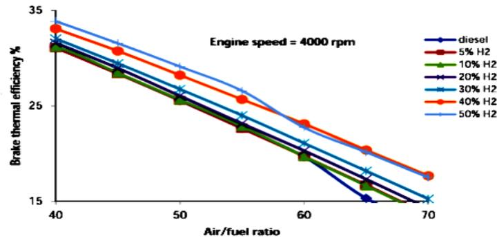
**Fig.1.Brake thermal efficiency vs A/F ratio for different H<sub>2</sub> concentration.**
